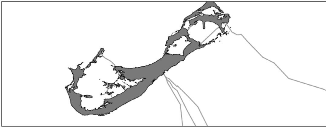
Figure 8.3.5. Exclusionary criteria were used to identify areas potentially suitable for renewable energy platform siting. Submarine cable routes are assumed to be unsuitable for energy platforms due to the need to access them, and the potential for damage during platform installation. This map shows cable route locations, as well as a 50 m buffer zone, i.e., areas to 50 m distance around the cables are excluded as suitable areas for energy platform siting.
